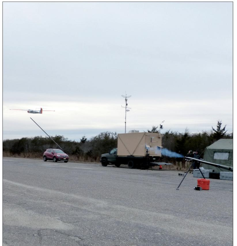
The drone, or Unmanned Aircraft System, as NJIT prefers to call it, takes off toward the ocean from a launcher using a pole and compressed air. The launcher allows the drone to use a smaller engine, which is not capable of providing enough power for takeoff.
